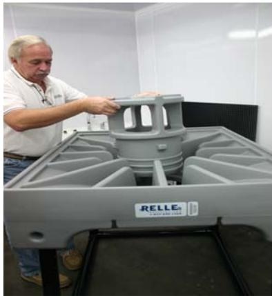
7. Place the table top grid into the top of the table. This grid is very fragile and proper handling must be utilized in order to prevent breakage of grid.
