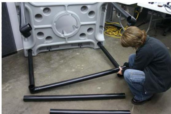
4. Connect the short cross braces (31") into the 3 way elbow to span the width of the table.
