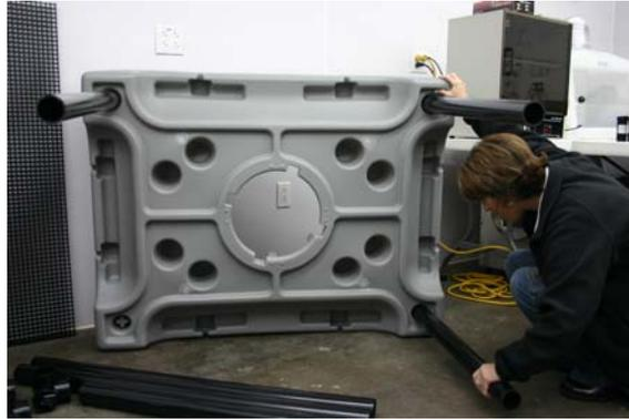
2. At the bottom of the legs insert the 3 way elbows. (It is recommended that all pieces inserted into 3 way elbow be glued in place using the proper ABS cement.)
